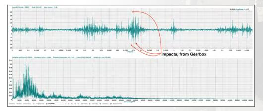
When running without load the amplitude was .3493 G's Overall RMS. As you can see above when the vibration is induced under load/cut it rises to 2.26 G's RMS and has peaks up to 25 G's.
